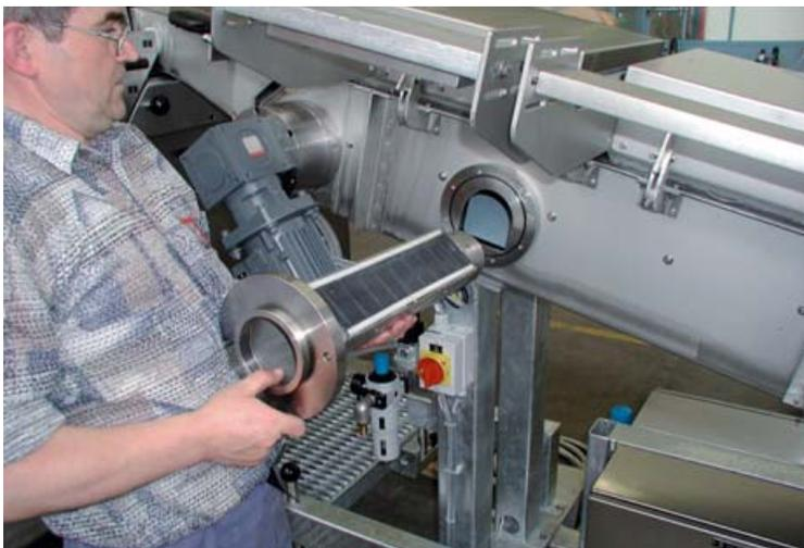
Variable positioning of the exhaust air nozzles
