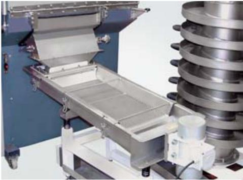
Classifier with spiral conveyor for downstream processing
